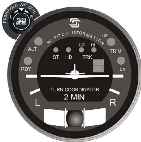
Fig. 2-11. AP Display, Turn Coordinator Failure (System Thirty)
