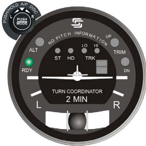
Fig. 2-10. AP Display, RDY for Operation (System Thirty)
