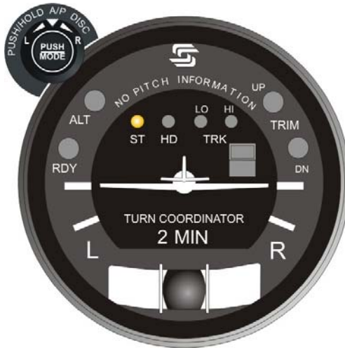
Fig. 3-1. AP Display, ST Mode Engaged
