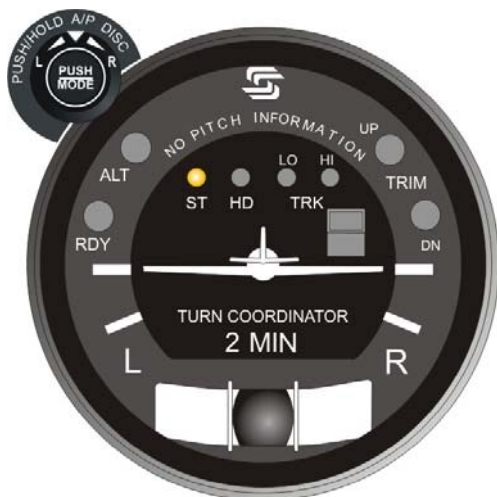
Fig. 2-21. AP Display, ST Mode Engaged (System Thirty)
