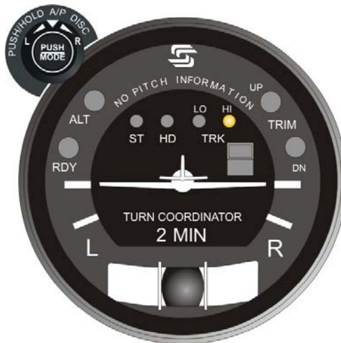
Fig. 3-4. AP Display, HI TRK Mode Engaged
