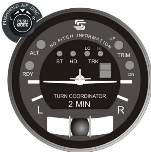
Fig. 2-9. AP Display, All Lamps Extinguished (System Thirty)
